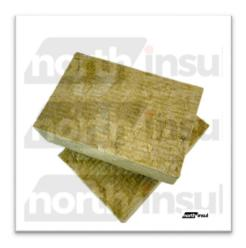
NI S40 - Safing Insulation is a lightweight, semi-rigid stone wool insulation board designed specifically for use in fire stopping applications. It can be used to fill perimeter gaps between concrete floor slabs and exterior wall systems. It can also be used to fill gaps in rated walls, floor/ceiling assemblies. It is also used in pipe and duct penetrations through walls and floor slabs.
